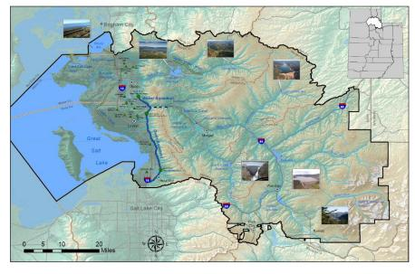
dam, then flows through the canal until it enters two large aqueducts along the Wasatch bench. Several creeks along the Wasatch Front can feed into this aqueduct system. From there, water is transported to each of the District's water treatment plants (WTPs). After complete treatment, water is delivered to cities or water improvement districts for final distribution to individual users.
